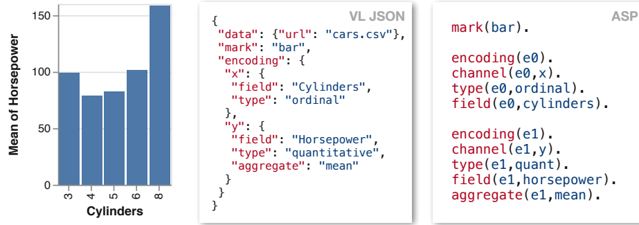
Figure 2.2: An example specification of a bar chart by VL and in the ASP notation resulting from Draco’s recommendation pipeline. It defines a mark type, two encodings and their field, data type, and data transformation definition - reprinted from Moritz [MWN + 19].
